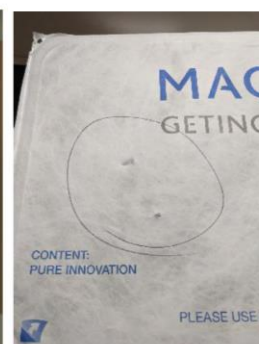
Figure 4: example of holes in the Tyvek cover
